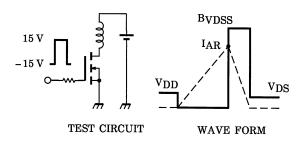
$$\begin{aligned} R_G &= 25~\Omega \\ V_{DD} &= 90~\text{V},~L = 7.35~\text{mH} \end{aligned} \quad E_{AS} &= \frac{1}{2} \cdot L \cdot I^2 \cdot \left( \frac{B\text{VDSS}}{B\text{VDSS} - \text{VDD}} \right) \end{aligned}$$
