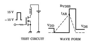
$$\begin{aligned} R_G &= 25~\Omega \\ V_{DD} &= 90~V,~L = 12.2~mH \end{aligned} \quad E_{AS} &= \frac{1}{2} \cdot L \cdot I^2 \cdot \left( \frac{BVDSS}{BVDSS - VDD} \right) \end{aligned}$$
