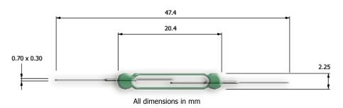
This reed switch is designed for performance at moderate inductive loads of 15W. The flattened lead outs are especially useful for orienting the internal blades to face one way while soldering, welding etc, for maximum in-group sensitivity. The three differential bands which are available cover a wide range of release specific applications. This reed switch is Lead (Pb) free and RoHS compliant.
