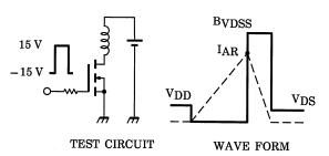
$$\begin{aligned} &R_G = 25 \ \Omega \\ &V_{DD} = 90 \ V, \ L = 43.6 \ mH \end{aligned} \quad EAS = \frac{1}{2} \cdot L \cdot I^2 \cdot \left( \frac{BVDSS}{BVDSS - V_{DD}} \right)$$
