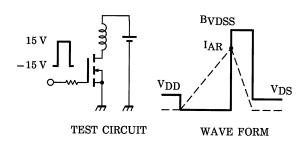
$$\begin{aligned} &RG = 25~\Omega \\ &V_{DD} = 90~V,~L = 17.4~mH \end{aligned} \quad E_{AS} = \frac{1}{2} \cdot L \cdot I^2 \cdot \left( \frac{BV_{DSS}}{BV_{DSS} - V_{DD}} \right) \end{aligned}$$
