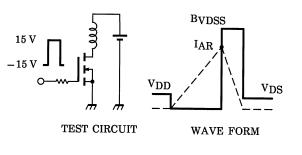
$$\begin{array}{l} \mathrm{R_{G}=25\ \Omega}\\ \mathrm{V_{DD}=90\ V,\ L=60\ mH} \end{array} \qquad \mathrm{EAS}=\frac{1}{2}\cdot\mathrm{L}\cdot\mathrm{I}^{2}\cdot\left(\frac{\mathrm{B}\mathrm{VDSS}}{\mathrm{B}\mathrm{VDSS}-\mathrm{V_{DD}}}\right) \end{array}$$
