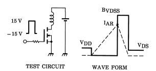
$$\begin{aligned} R_G &= 25~\Omega \\ V_{DD} &= 50~V,\, L = 1.48~mH \end{aligned} \qquad EAS = \frac{1}{2} \cdot \end{aligned}$$
