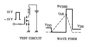
$$\begin{aligned} R_G &= 25~\Omega \\ V_{DD} &= 25~V,~L = 440~\mu H \end{aligned} \qquad EAS &= \frac{1}{2} \cdot L \cdot I^2 \cdot \left( \frac{BVDSS}{BVDSS - VDD} \right) \end{aligned}$$
