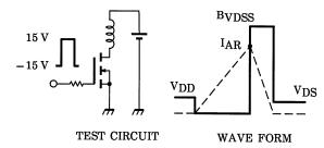
$$\begin{aligned} &R_G = 25~\Omega \\ &V_{DD} = 25~V,~L = 471~\mu H \end{aligned} \qquad EAS = \frac{1}{2} \cdot L \cdot I^2 \cdot \left( \frac{BVDSS}{BVDSS - VDD} \right)$$
