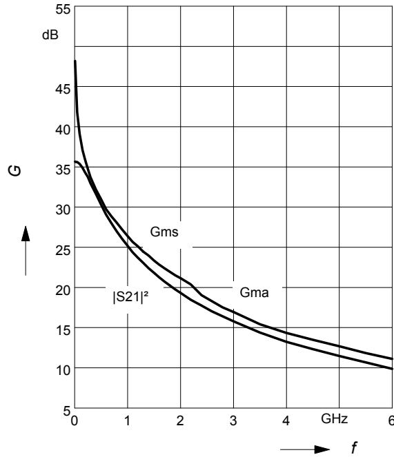
**Power gain  $G_{ma}$ ,  $G_{ms} = f(V_{CE})$**
