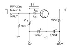
I<sub>C</sub>=20I<sub>B1</sub>=-20I<sub>B2</sub>=300mA (For PNP, the polarity is reversed)
