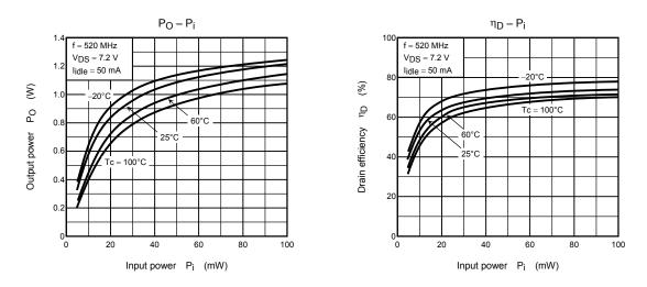
Note 3: These are only typical curves and devices are not necessarily guaranteed at these curves.
