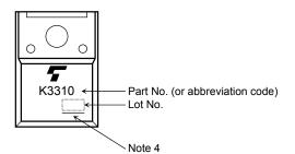
Note 4: A line under a Lot No. identifies the indication of product Labels. Not underlined: [[Pb]]/INCLUDES > MCV Underlined: [[G]]/RoHS COMPATIBLE or [[G]]/RoHS [[Pb]]
