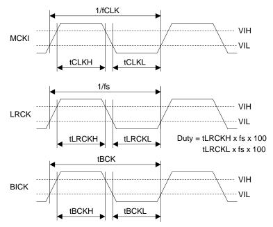
Figure 12. Clock Timing (EXT Slave mode)
