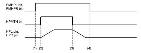
Figure 52. Power-up/Power-down Timing for Headphone-Amp
