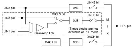
Figure 56. HPL Mixing Circuit (AIN3 bit = "1", HPG bit = "0")
