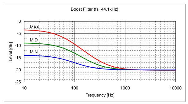
Figure 35. Bass Boost Frequency Response (fs=44.1kHz)
