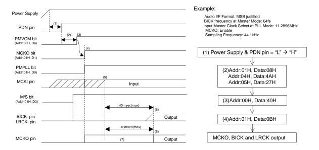
Figure 74. Clock Set Up Sequence (1)
