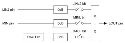
Figure 44. LOUT Mixing Circuit (AIN3 bit = "0", LOVL bit = "0")
