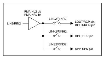
Figure 38. Analog Mixing Circuit (LIN2/RIN2)
