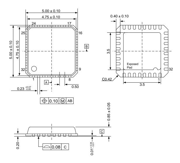
Note) The exposed pad on the bottom surface of the package must be open or connected to the ground.
