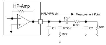
Figure 2. Headphone-Amp output circuit
