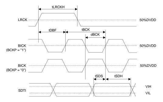
Figure 5. Audio Interface Timing (PLL/EXT Master mode, DSP mode, MSBS = "1")
