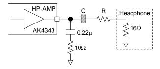
Figure 53. External Circuit Example of Headphone
