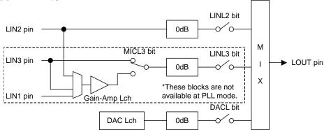
Figure 46. LOUT Mixing Circuit (AIN3 bit = "1", LOVL bit = "0")
