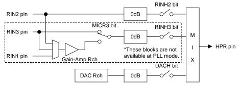
Figure 57. HPR Mixing Circuit (AIN3 bit = "1", HPG bit = "0")
