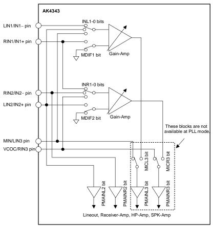
Figure 37. Analog Mixing Circuit
