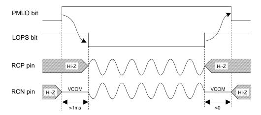
Figure 49. Power-up/Power-down Timing for Receiver-Amp
