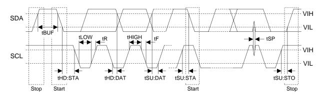
Figure 16. I<sup>2</sup>C Bus Mode Timing
