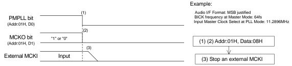
Figure 84. Clock Stopping Sequence (1)
