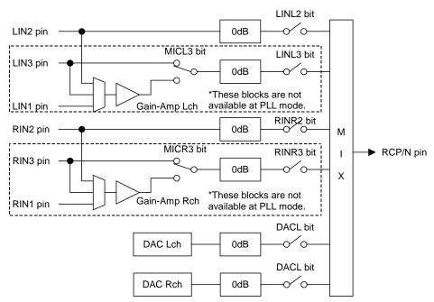
Figure 51. Receiver Mixing Circuit (AIN3 bit = "1", LOVL bit = "0")
