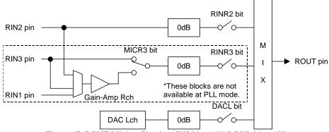
Figure 47. ROUT Mixing Circuit (AIN3 bit = "1", LOVL bit = "0")
