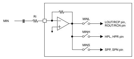
Figure 40. Block Diagram of MIN pin
