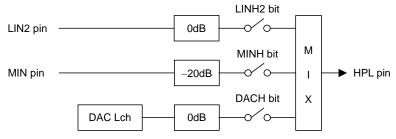
Figure 54. HPL Mixing Circuit (AIN3 bit = "0", HPG bit = "0")
