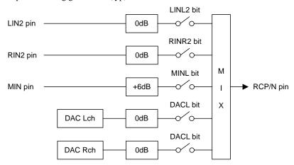
Figure 50. Receiver Mixing Circuit (AIN3 bit = "0", LOVL bit = "0")
