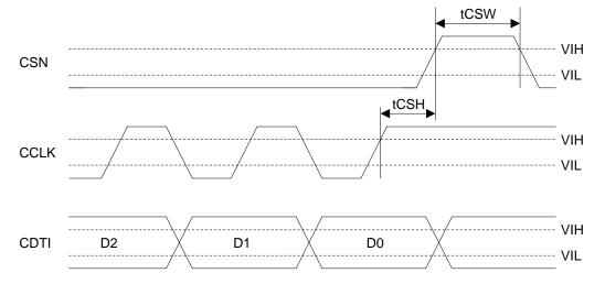
Figure 15. WRITE Data Input Timing
