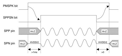
Figure 59. Power-up/Power-down Timing for Speaker-Amp
