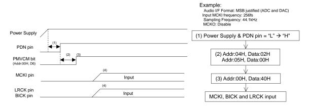
Figure 77. Clock Set Up Sequence (4)
