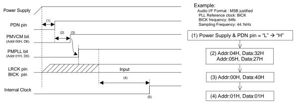
Figure 75. Clock Set Up Sequence (2)
