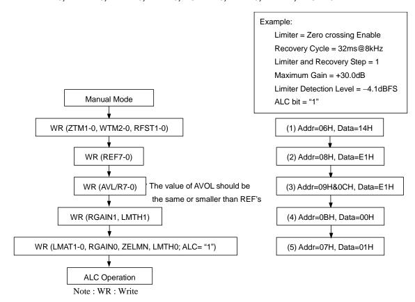
Figure 33. Registers set-up sequence at ALC operation
