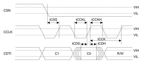
Figure 14. WRITE Command Input Timing
