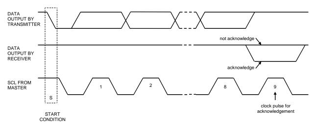
Figure 70. Acknowledge on the I<sup>2</sup>C-Bus
