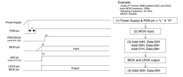
Figure 78. Clock Set Up Sequence (5)
