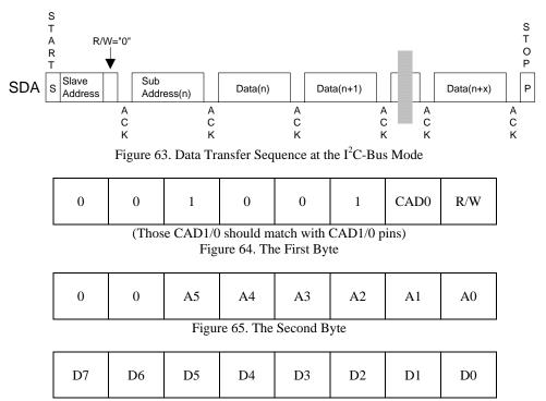
Figure 66. Byte Structure after the second byte
