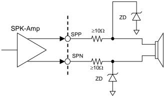
Figure 58. Speaker Output Circuit (Load Capacitance > 30pF)
