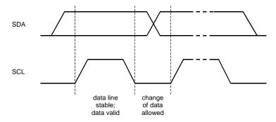
Figure 71. Bit Transfer on the  $I^2C$ -Bus
