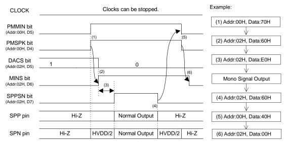
Figure 80. "MIN-Amp → Speaker-Amp" Output Sequence
