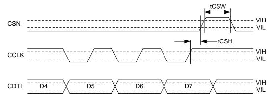
Figure 4. WRITE Data Input Timing
