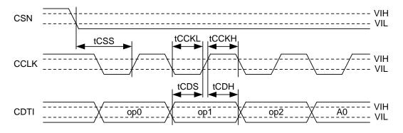
Figure 3. WRITE Command Input Timing
