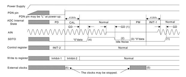
Figure 8. Power up / Power down Timing Example
