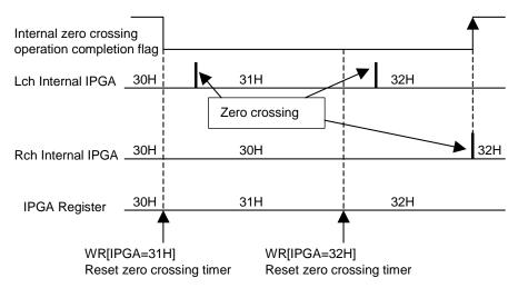
Figure 11. About Zero Crossing Operation
