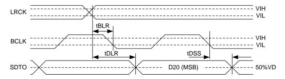
Figure 2. Audio Data Input/Output Timing (Audio I/F = No.0)
