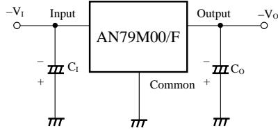
C<sub>I</sub> is connected when the input line is long. 2μF
