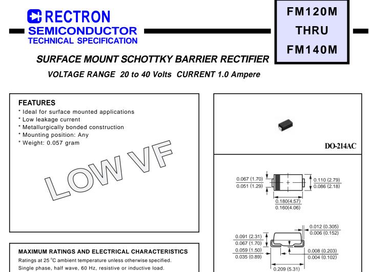
Single phase, half wave, 60 Hz, resistive or inductive load. For capacitive load, derate current by 20%.
