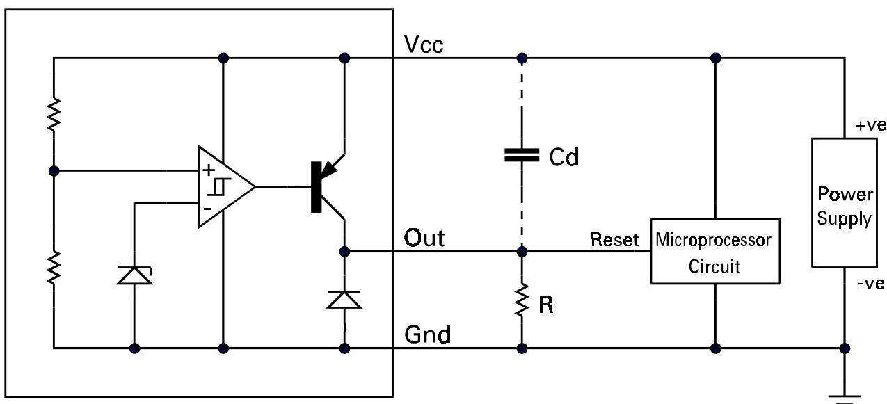
Note 4: A time delayed reset can be accomplished with the additional Cd.
