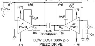
Two PA241 amplifiers operated as a bridge driver for a piezo transducer provides a low cost 660 volt total drive capability. The R<sub>N</sub> C<sub>N</sub> network serves to raise the apparent gain of A2 at high frequencies. If R<sub>N</sub> is set equal to R the amplifiers can be compensated identically and will have matching bandwidths.
