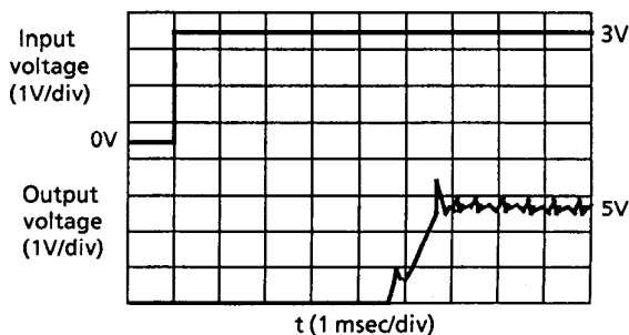
S-8322AA V_{IN} = 0 \rightarrow 3\text{V} , R_L = 250\Omega
