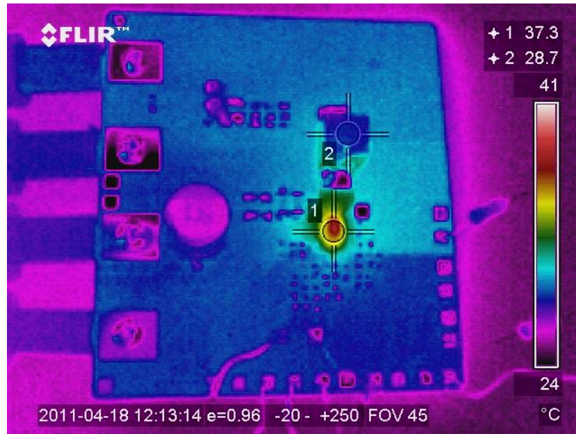
Figure 42: Thermal Image of the Board at 4A Load, Test Point 1 is IR3897, Test Point 2 is inductor
