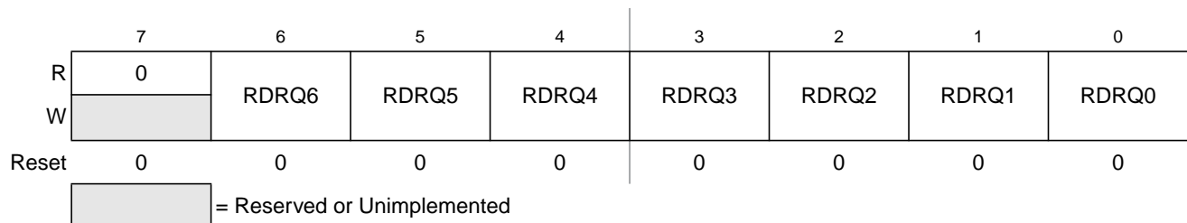
Figure 3-26. Port Q Reduced Drive Register (RDRQ)
