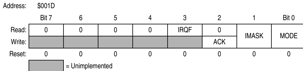
Figure 8-3. IRQ Status and Control Register (INTSCR)
