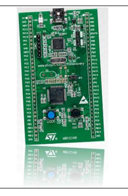
A large number of free ready-to-run application firmware examples are available on www.st.com/stm32f0discovery to support quick evaluation and development.
