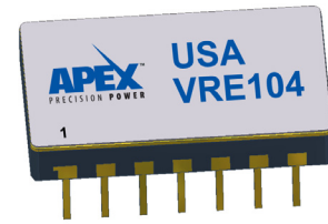
Hermetic 14-pin Ceramic DIP Package Style HC
