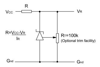
This circuit will allow the reference to be trimmed over a wide range. The device is specified over a  $\pm$ 5% trim range.
