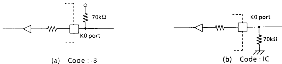
Figure 2. I/O code and external circuitry
