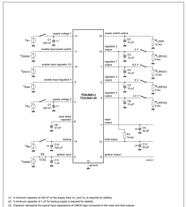
Fig.10 Test circuit of TDA3681J and TDA3681JR.
