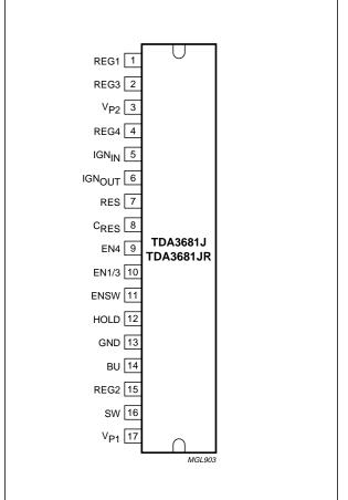
Fig.3 Pin configuration for TDA3681J and TDA3681JR.
