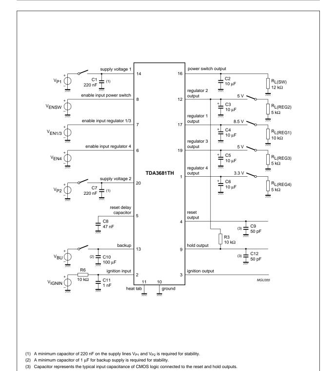
Fig.11 Test circuit of TDA3681TH.
