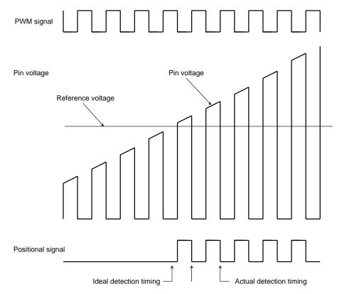
$\label{eq:lambda} \begin{array}{ll} \mbox{Variation is calculated through detection at two consecutive rising edges of the PWM signal.} \\ \mbox{1/f}_p < \mbox{Detection time variation} < 2/f_p & f_p \mbox{: PWM frequency.} \end{array}$
