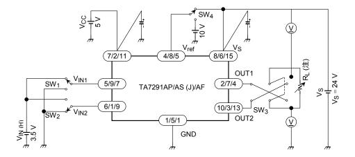
Note 1:  $I_{OUT}$  calibration is required to adjust specified values of test conditions by  $R_L$ . ( $I_{OUT} = 0.2 \text{ A}/0.4 \text{ A}/0.5 \text{ A}/1.0 \text{ A}$ )
