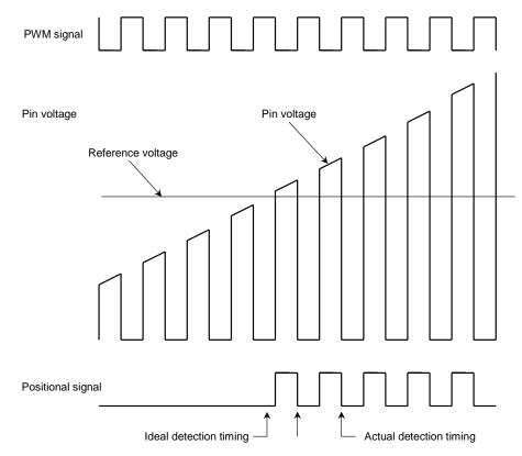
Variation is calculated by detecting at two consecutive rising edges of PWM signal.  $1/f_p < Detection time variation < 2/f_p$  fp: PWM frequency
