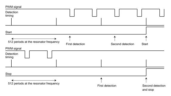
Note: Take sufficient care for noise on PWM signal input pin.
