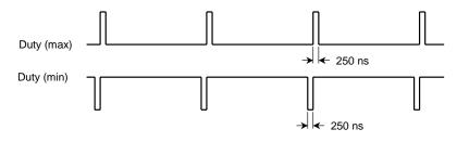
The voltage applied to the motor is duty 100% because of the storage time of the drive circuit even if the duty is 99%.
