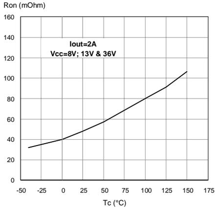
On State Resistance Vs  $V_{CC}$
