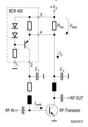
Be aware that BCR400 stabilized bias current of transistors in an active control loop
