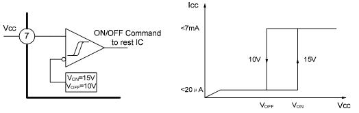
During Under-Voltage Lockout, the output driver is biased to a high impedance state. Pin6 should be shunt to GND with a bleeder resistor to prevent activing the power switch with output leakage currents.
