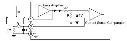
Peak current (I<sub>S</sub>) determined by the formula:  $I_{SMAX}$ =1V/Rs. A small RC filter be required to suppress switch transients
