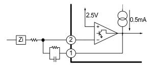
Error amplifier can source or sink up to 0.5mA
