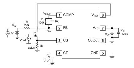
High peak current associated with capacity loads necessitate careful grounding techniques. Timing and bypass capacitors should be connected close to pin5 in single point GND.
