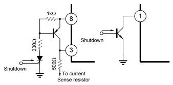
Shutdown UTC UC3842G can be accomplished by two methods; either raise pin 3 above 1V or pull Pin 1 below a voltage two diode drops above ground.
