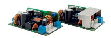
The new TOP-100 Series AC/DC Power Supplies feature the highest power rating in the industry standard  $2.0'' \times 4.0''$  (50.8 x 101.6 mm) footprint. They can supply up to 100 W output power with convection cooling over an industrial operating temperature range of  $-25^{\circ}$ C to  $+50^{\circ}$ C. This performance could be realized by a state of the art design providing an extremely high efficiency of >90 % which eliminates the need for a dedicated power supply cooling fan.
