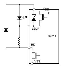
The type of relay should be normally closed (NC). A NC relay is opened by applying the control voltage on its coil and in this case the module is in Auto Shut-Off mode.
