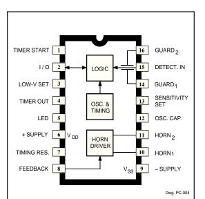
The A5349CA is a low-current, CMOS circuit providing all of the required features for an ionization-type smoke detector. A networking capability allows as many as 125 units to be interconnected so that if any unit senses smoke, all units will sound an alarm. In addition, special features are incorporated to facilitate alignment and test of the finished smoke detector. This device is designed to comply with Underwriters Laboratories Specification UL217.
