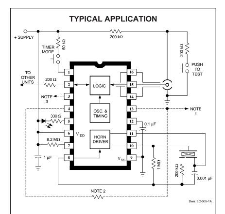
NOTE 1: Use an external resistor to adjust sensitivity for a particular smoke chamber.
