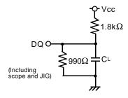
Fig.1 Output load
