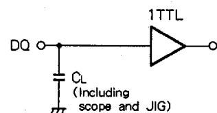
Fig.1 Output load
