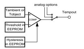
The comparator is a digital comparator, with a resolution of 12 bits. By default the input polarity is inverting. The default threshold and hysteresis values are version dependent, as indicated below.
