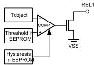
The comparator is a digital comparator, with a resolution of 12 bits. By default the input polarity is inverting. By default the trigger temperature is the object temperature but also the ambient (sensor) temperature can be used. Threshold and hysteresis values are version dependent, as indicated below.
