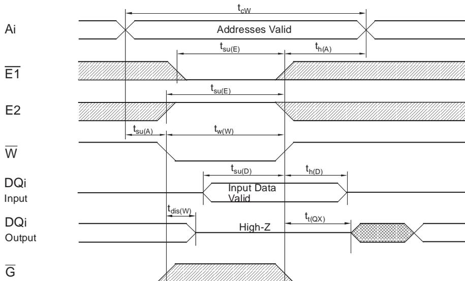
Write Cycle 2 ( $\overline{E1}$ -controlled)
