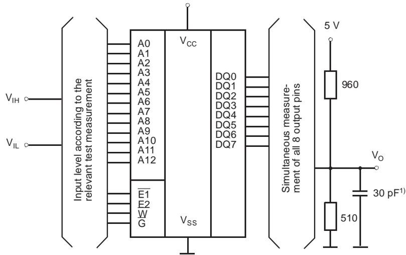
1) In measurement of  $t_{dis(E)}$ ,  $t_{dis(W)}$ ,  $t_{dis(G)}$  the capacitance is 5 pF.
