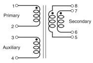
Secondary windings to be connected in parallel on PC board.
