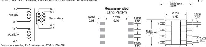
and FCT1-150K2SL. For other parts, secondary windings to be connected in parallel on PC board.
