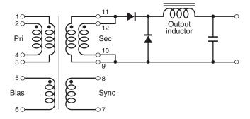
The primary windings and the secondary windings are to be connected in parallel on the PC board.
