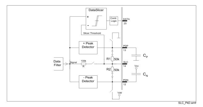
Figure 3-23 Slicer Level using Peak Detector
