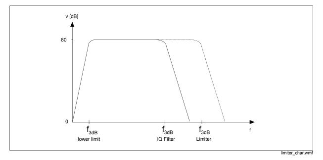
Figure 3-20 Limiter frequency characteristics
