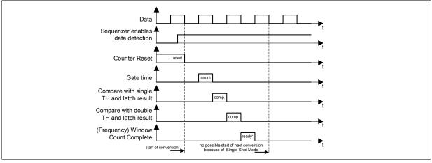
Timing in Single Shot mode can be seen in the subsequent figure:
