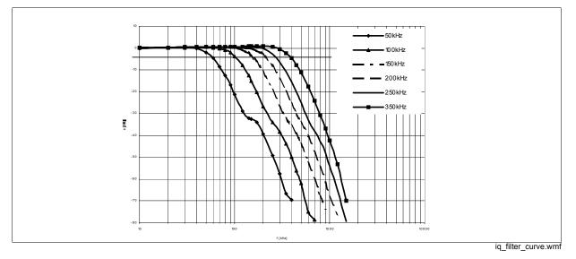
Figure 3-17 I/Q Filter Characteristics
