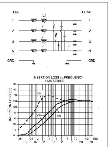
The 1138 series is a 3 phase WYE filter. This series is designed to be used with military systems which are requires to meet the conducted emissions of MIL STD - 461C / CE03.
