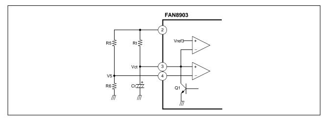
If the up/down switch is pushed less than a set time ( $T_s$ ), TR (Q1) will be turned off and capacitor (Ct) is charged exponentially until Vct equals to V5. At that time TR (Q1) is turned on and stops the operation.
