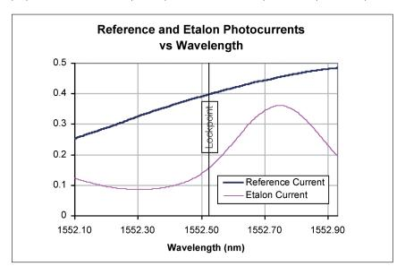
In order to lock the LMC10NEG wavelength, a control circuit should be used which maintains the laser submount temperature constant over life and then controls the wavelength by varying the laser forward current to keep the ratio of the etalon and reference photodiode currents (Locking Ratio) constant. This may be achieved by keeping the discrimination value (LR x  $I_{ref}$ ) –  $I_{et}$ ) at zero, where LR is the target Locking Ratio.
