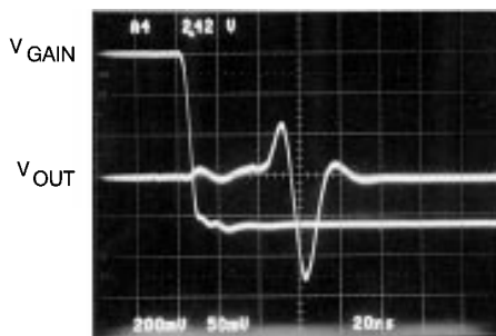
V_{GAIN} Overload Recovery Response—No AC Input
