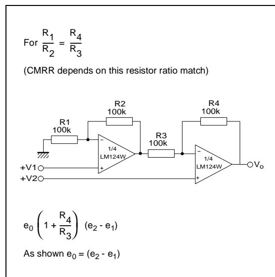
**USING SYMETRICAL AMPLIFIERS TO REDUCE INPUT CURRENT (GENERAL CONCEPT)**
